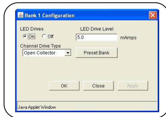
Figure 4-5. The Bank (Distribution Board) Configuration Window.
